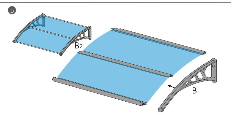
Place the holder (B) on the roof plates (A)
