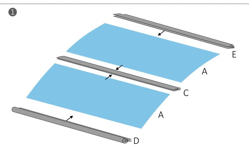
Place the roof plates (2XA) on the connection profile (C) and a front profile (D) a wall profile (E)
