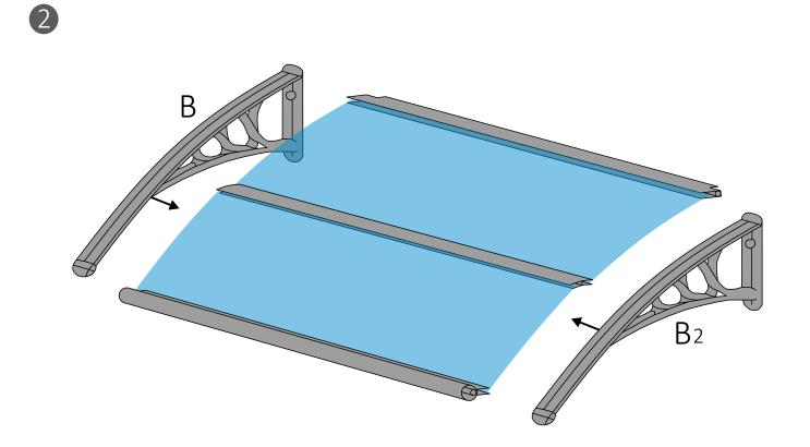
Place the holder (B) and (B2) on the roof plates (A)
