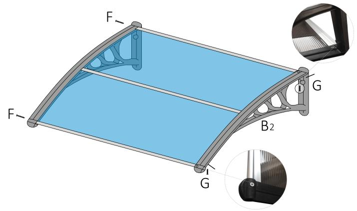
Attach the holder (B) to the front profile (D) and the Wall profile (E) by screws (F) and the inner holder (B2) by screws (G) from the bottom to the front profile (D) and the Wall profile (E)
