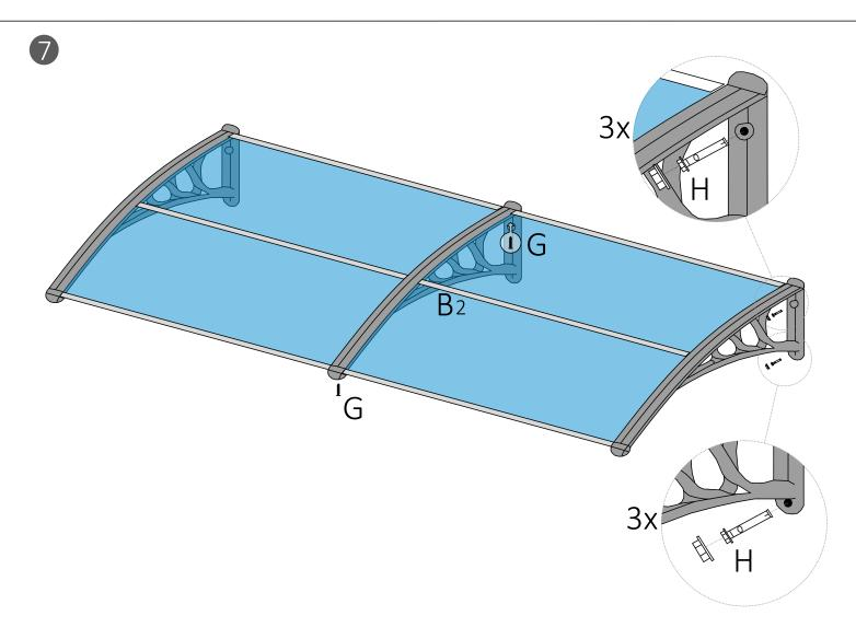
Fasten the inner holder (B2) by screws (G) from the bottom to the front profile (D) and the Wall profile (E)
