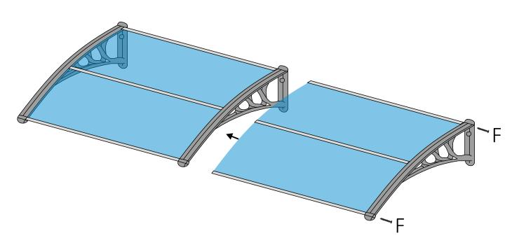
Fasten the holder (B) by screws (F) to the front profile (D )and wall profile (E ) and place the second part of the canopy on the first part
