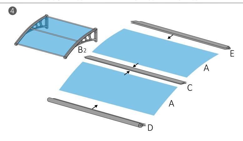
Place the roof plates (2XA) on the connection profile (C) and a front profile (D) a wall profile (E)
